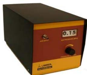
To supply vacuum or compressed air, e.g. for the aeration of fermenters and bioreactors in biotechnological laboratories not equipped by central air and vacuum lines, LAMBDA has developed an innovative, microprocessor controlled, compact and virtually noiseless air compressor and vacuum pump – the LAMBDA AeroSilento.
