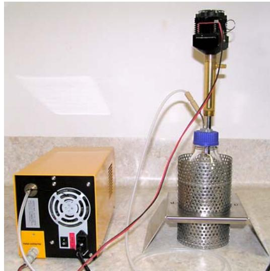
8. Connect the Peltier cooling trap to the corresponding socket on the rear of the AeroSilento air compressor.
